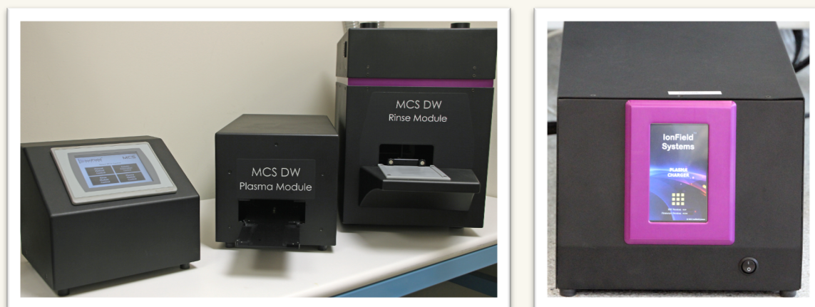
PurePLATE MCS Components: Plasma Module, Rinse Module, Communication Module and PlasmaCharger
